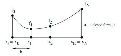
• Note that for Newton-Cotes formulae only the weighting coefficients  $w_i$  were unknown and the  $x_i$  were fixed
