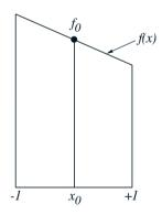
• We can integrate exactly with only 1 point for a linear function while for Newton-Cotes we needed two points!
